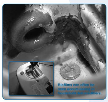
Biofilm thickness is variable but is usually in the range of 50 to 100 microns. As the thickness increases, pieces of biofilms can shear off, allowing for colonization of downstream sections of the system.
