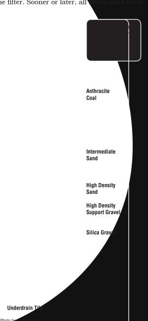
gets clogged, more negative pressure is created. The pressure usually starts near zero pounds per square inch (psi) or approximately one foot of head loss on the clean filter. Then the pressure will increase in a linear fashion in the negative direction to approximately -2.5 to -4 psi on rapid-rate, gravity filters and
