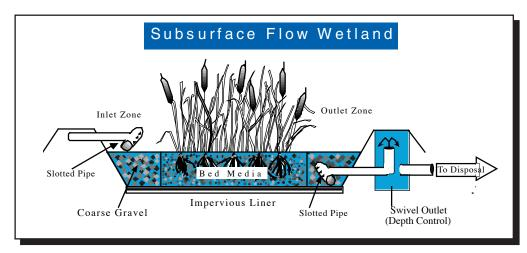
In the U.S., gravel and rock are the most common media used in subsurface flow wetlands. Whatever type or size media material is chosen, the most important concern is that it be as uniform in size as possible. When different size media are placed together in systems, the result is fewer spaces between the media, and finer materials settle into the remaining spaces, leaving little room in the system for the wastewater to flow.
