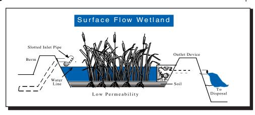
account when designing wetland systems. In addition, they usually size surface flow systems generously as a precaution to ensure that treatment standards are always met, even in the face of such unforeseeable events as unusually prolonged periods of rain or extreme cold.
