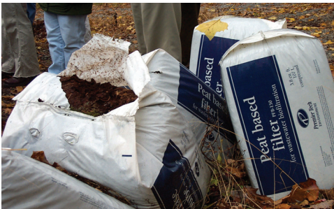
Bags of peat moss ready for installation in a filter
